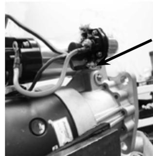
Remove relay nut and ring terminal. Relay nut can be either 8mm or 10mm depending on model.
