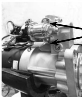
Remove relay mounting screws
